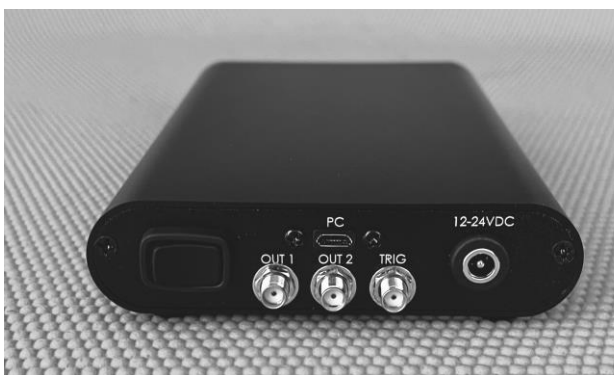
Interrogator rear panel view
